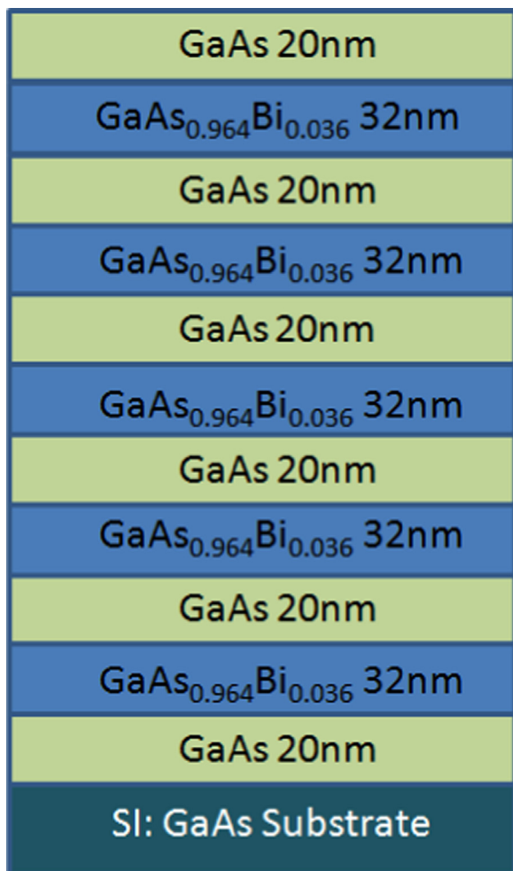
Fig. 1. Structure details for the samples employed in the annealing study. GaAs was grown at 650 °C while \text{GaAs}_{0.964}\text{Bi}_{0.036} was grown at 380 °C. Bi mole fraction is an average value in a \text{GaAs}_{1-x}\text{Bi}_x layer deduced from the HR-XRD measurement.
