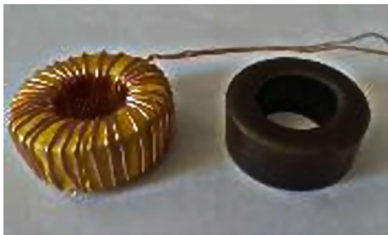
Fig. 1. Samples of FeSiAl magnetic powder cores.
