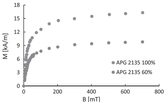
**Fig. 1.** Magnetization curves for the diluted and non-diluted samples, the curves exhibit identical characteristics except for a scaling factor of 0.6 that reflects the different concentrations of nanoparticles.
