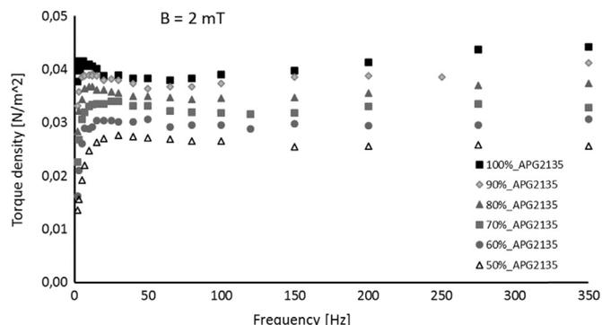
**Fig. 3.** Experimental torque densities versus rotation frequency at a magnetic field of 2 mT.
