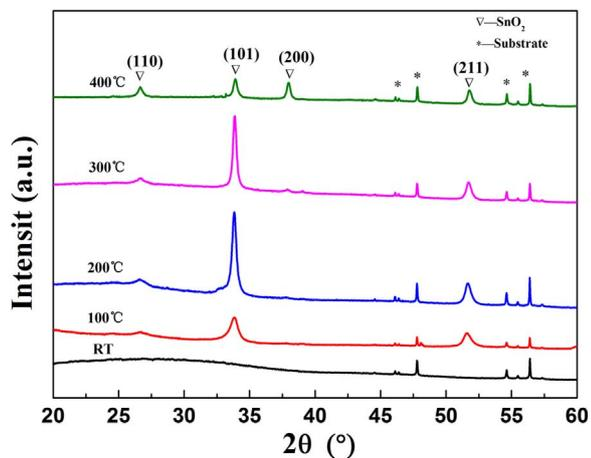
Fig. 1. XRD data of the SnO<sub>2</sub> films grown at temperatures ranged from room temperature to 400 °C.
