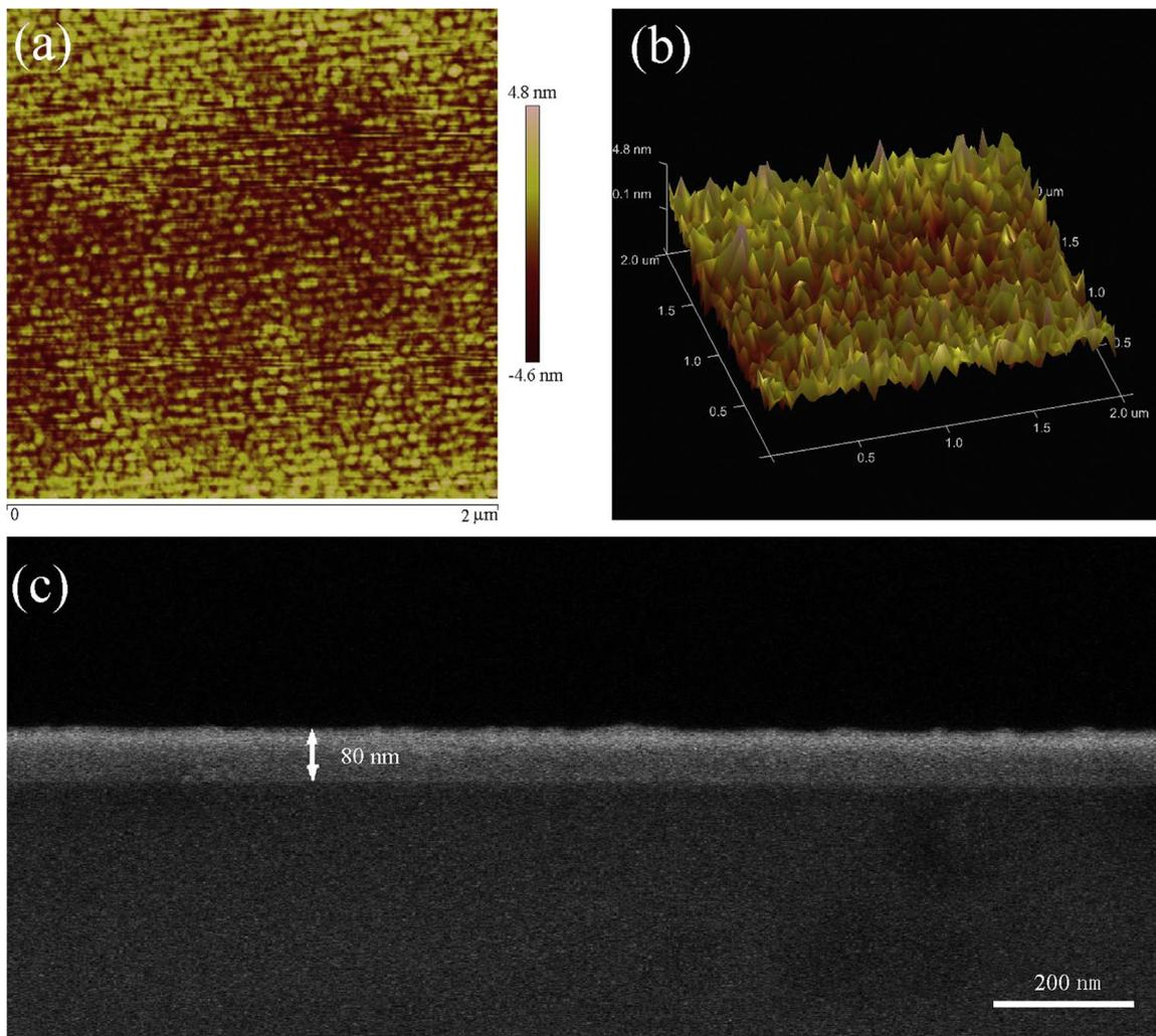
Fig. 2. Typical AFM images showing the surface (a) morphology and (b) roughness of the SnO<sub>2</sub> film. (c) Cross sectional SEM image demonstrating the thickness of the film.
