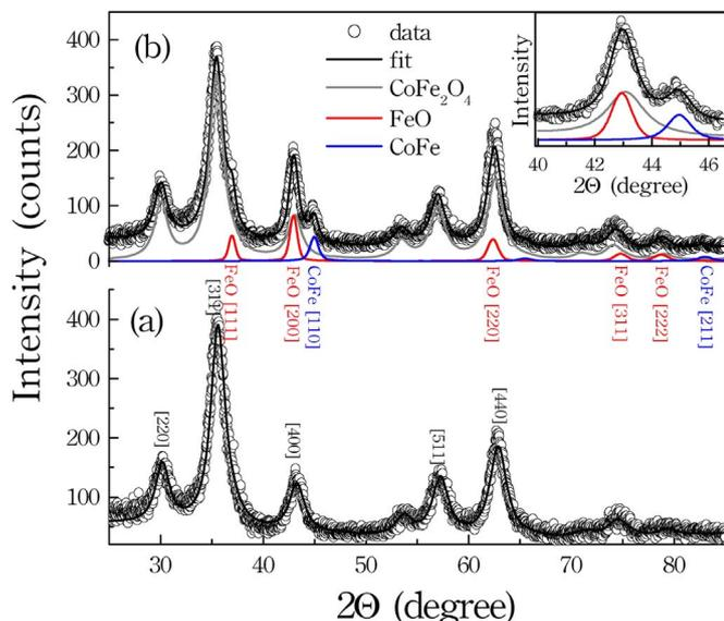
**Fig. 1.** X-ray diffractograms for pure  $\text{CoFe}_2\text{O}_4$  (a) and for  $\text{CoFe}_2\text{O}_4/\text{CoFe} - \text{FeO}$  (b). All the peaks observed by XRD were properly indexed by using the three proposed crystalline phases. The open circles are experimental data and the solid lines are fits obtained by Rietveld refinement. The inset in Fig. 1(b) is a blow-up for  $2\theta$  in the range 40–47.
