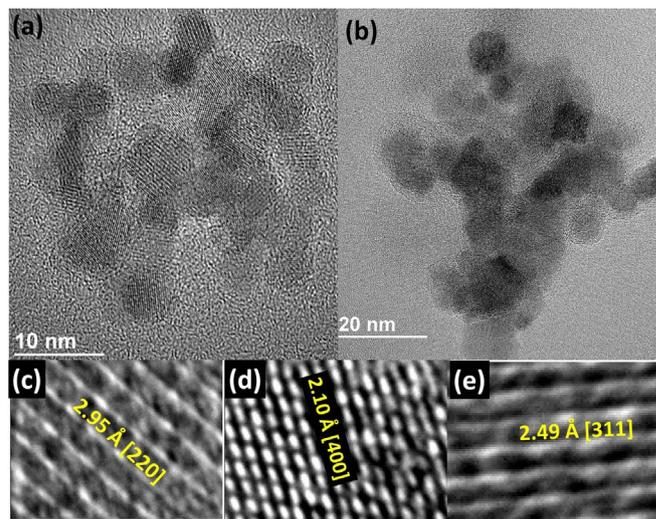
**Fig. 2.** TEM images for (a)  $\text{CoFe}_2\text{O}_4$  and for (b)  $\text{CoFe}_2\text{O}_4/\text{CoFe} - \text{FeO}$ . Details of the first layers were also obtained by using high resolution TEM for a nanoparticle of  $\text{CoFe}_2\text{O}_4$  (c–e).
