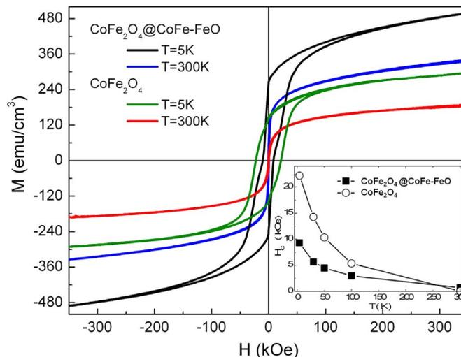
**Fig. 3.** Hysteresis loops for  $\text{CoFe}_2\text{O}_4$  and for  $\text{CoFe}_2\text{O}_4/\text{CoFe} - \text{FeO}$ , for  $T = 5$  and 300 K. The inset shows the  $T$ -dependence of the coercive field  $H_c$  for both samples.
