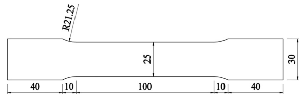
Fig. 1. Shape and dimensions of specimens (unit: mm).
