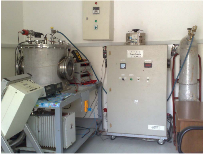
Fig. 1. DC-sputtering device set up for preparing NiO thin films.
