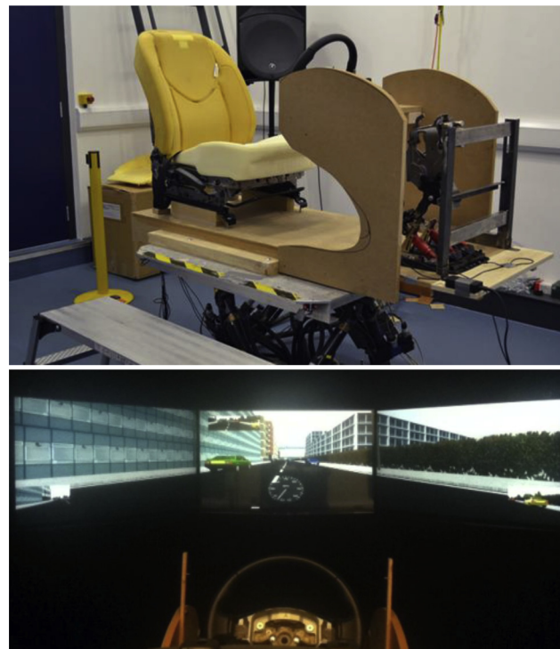
Fig. 1. Laboratory set up including driving rig, seat, steering wheel, pedals and driving simulator.
