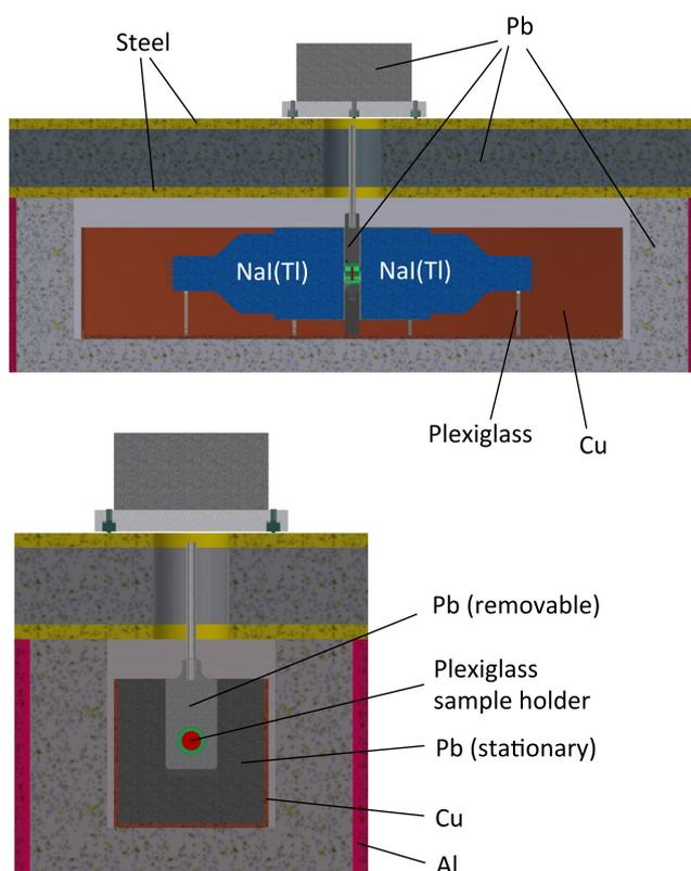
Fig. 2. (Color online) Cross-sectional views of the  $\gamma\gamma$ -coincidence spectrometer, showing the geometry and the different layers of materials. Part of the lead shield, located between the two detectors (see lower panel), was removable and contained the sample holder made of plexiglass.
