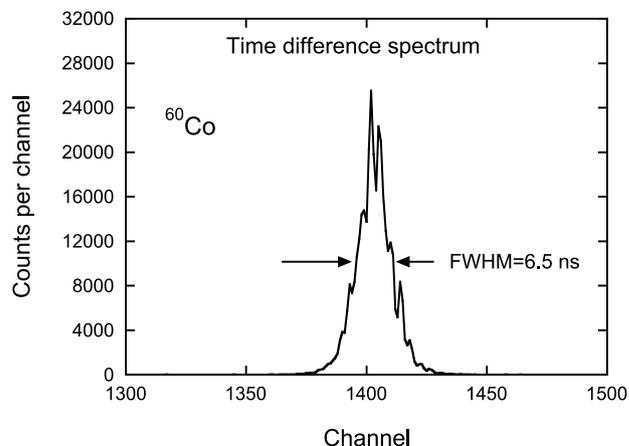
Fig. 3. Timing spectrum of the NaI(Tl)  $\gamma\gamma$ -coincidence spectrometer, measured using a  $^{60}\text{Co}$  calibration source. A 13-ns wide software gate around this peak defined a coincidence event between the two detectors. Additional coincidence gates were applied to certain energy regions (see text).
