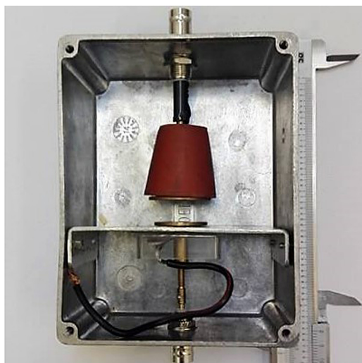
Fig. 1. Frontal view of the IC. During measurements, the IC is closed by putting the aluminium cover on the front face of the chamber.
