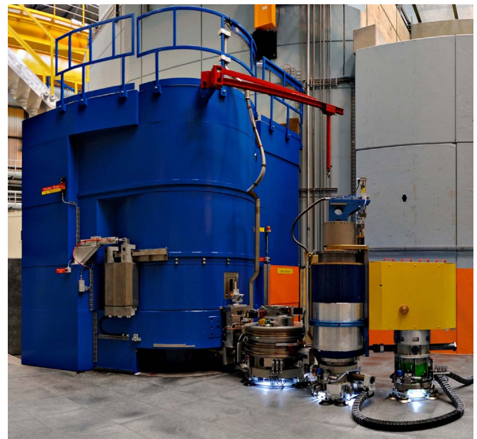
Fig. 3. Picture of the monochromator shielding, sample table and the secondary spectrometer with the analyzer housing and the detector shielding of EIGER.
