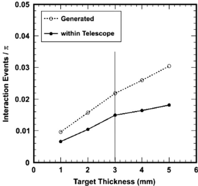
Fig. 2. Simulation results of the ratio of incident pions that interact with the copper target and the total amount of pions in function of the target thickness. The dashed line corresponds with the total amount of interactions and the solid line with those whose trajectory is within the telescope acceptance.
