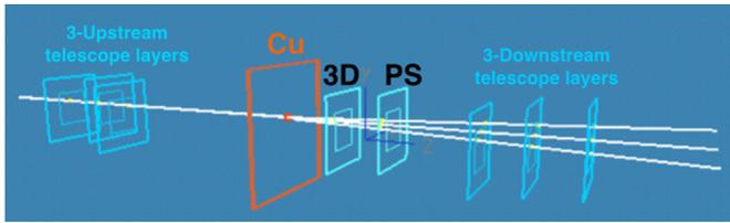
Fig. 1. Schematics of the experiment carried out. From left to right: 3 upstream telescope layers, copper target, 3D pixel sensor, planar sensor and the 3 downstream telescope layers.
