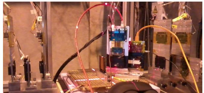
Fig. 4. Picture of the experiment setup along the beam line. The telescope, target and devices under test are visible.
