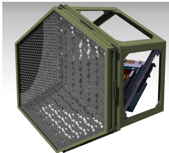
Fig. 1. Rendering of the camera structure. The PDP backplate is clearly visible together with some of the modules installed on it and the window covering them. On the back the 3 DigiCam micro-crates are visible.
