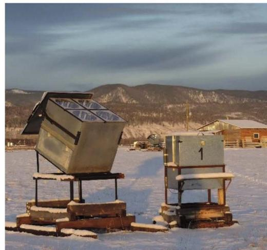
Fig. 1. Station layout of the TAIGA-HiSCORE array. Left: Location of the 28 optical stations (square) in the inner part of Tunka-133 Cherenkov light detectors (circles). Right: Photo of the optical station and its electronic box. In the background – the central DAQ building.
