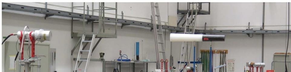
**Fig. 1.** The irradiation setup of the EJ-301 detector (left) corresponding to the  $0^\circ$  orientation in Table 1. The shadow cone is visible toward the right. The neutron beam enters the setup from the right.
