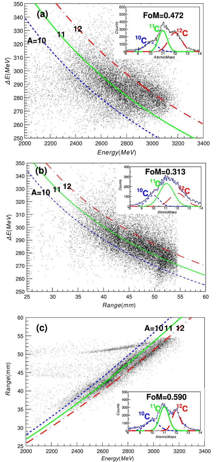
Fig. 2. The PID spectra for carbon isotopes obtained from Monte Carlo simulation with 2% energy resolution for each layer of the telescope. (a) The PID spectrum using the  $\Delta E - E$  method, (b) is the PID spectrum through the  $\Delta E - \text{Range}$  method, and (c) is the PID spectrum through the  $\text{Range} - E$  method. The FoM are calculated for  $^{11}\text{C}$  and  $^{12}\text{C}$ .
