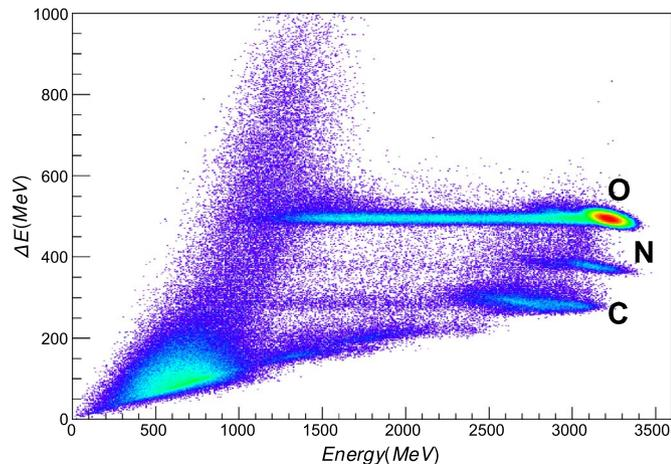
Fig. 1. The  $\Delta E - E$  PID spectra of the detector obtained from Monte Carlo simulation with 2% energy resolution for each layer of the telescope.
