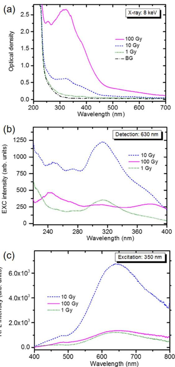
Fig. 1. Steady-state absorption spectra including BG spectra (a) as well as excitation spectra (b) and emission spectra (c) of Ag-glass after X-ray irradiation at various doses.
