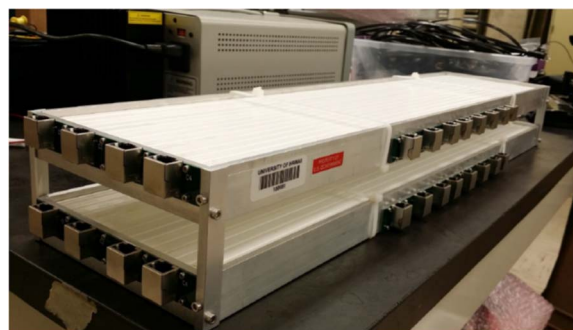
Fig. 1. Prototype BMD assembly showing layers of polystyrene rods and SiPM photodetector assemblies.
