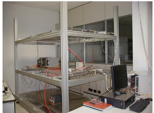
Figure 1: One EEE telescope composed of three MRPC chambers.
