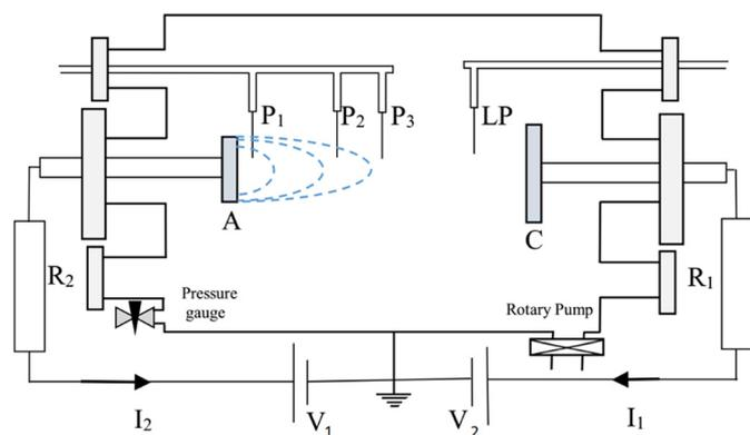
**Fig. 1.** Schematic of the experimental setup. A typical ADL profile with concentric DL structure is schematically shown in front of the anode.  $V_1$  and  $V_2$  = DC power supplies,  $A$  = anode,  $C$  = cathode,  $R_1$  and  $R_2$  = current limiting resistor,  $I_1$  and  $I_2$  = current measured through  $R_1$  and  $R_2$ .  $P_1$ ,  $P_2$  and  $P_3$  = floating probes.  $P_L$  = Langmuir probe.
