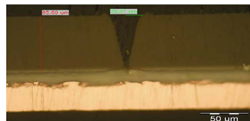
Fig. 3. Cross-section of ‘V’ form bending window, where the cut almost reached the copper layer.
