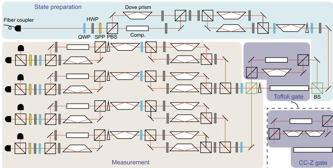
Fig. 2. (Color online). Proposal of experimental setup. The blocks with different colors represent the different basic stages. State preparation (blue block): three qubit encoding setup. Toffoli gate (purple block): Toffoli gate operating setup. CCZ gate (purple block): CCZ gate operating setup. Measurement (yellow block): qubit measuring setup.
