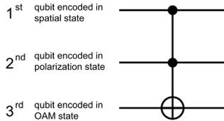
Fig. 1. Quantum Toffoli gate for three qubits encoded into three DOFs of a single photon.
