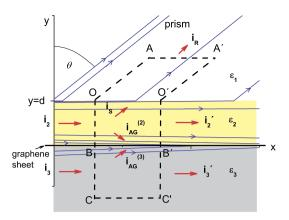
**Fig. 1.** (Color online.) Schematic illustration of the ATR geometry. The graphene sheet is located at y = 0 interface, between media 2 and 3. Closed region where energy conservation is applied (dashed line). Lines of Poynting vector flux are plotted (blue lines) for  $\omega/c = 0.025 \ \mu m^{-1}$  and thickness  $d = 0.026\lambda$ .  $\varepsilon_1 = 16$ ,  $\varepsilon_2 = 1$ ,  $\varepsilon_3 = 3.9$  and graphene parameters are  $\mu_c = 0.35$  eV,  $\gamma = 0.1$  meV and T = 300 K.
