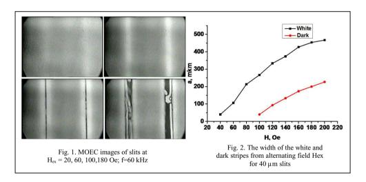
With increasing  $H_{ex}$ , size of all strips images is increasing. As it is seen from Fig. 2 the size of white and dark MO images significantly exceed the physical size of the gaps by 12 and 6 times, accordingly.
