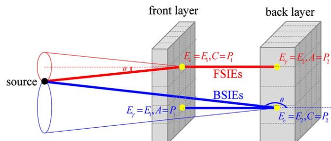
Fig. 1. Schematic of a Compton imager comprising two layers of CdZnTe pixel array detectors. (For interpretation of the references to color in this figure legend, the reader is referred to the web version of this article).
