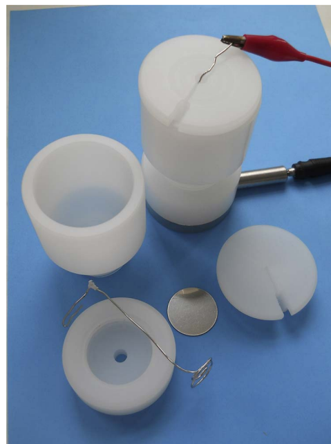
Fig. 1. Photography of the polypropylene electroplating cell manufactured at Jožef Stefan Institute, Ljubljana, Slovenia.
