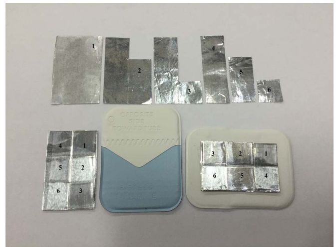
Fig. 1. Layout and position of Al filters on E speed Kodak dental film.
