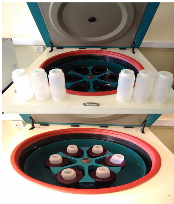
Fig. 1. Multipurpose Centrifuge machine having maximum capacity of 6 numbers of 500 mL centrifuge bottle.
