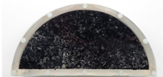
Fig. 1. A photo of the physical breast phantom, filled with water.
