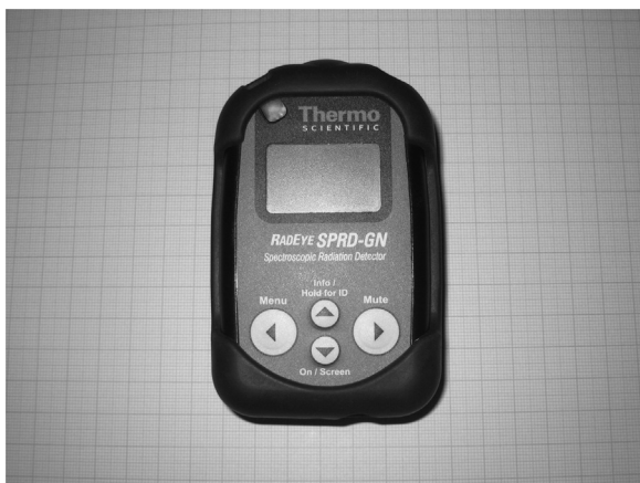
Fig. 1. Experimental CLYC dosimeter, using the hardware of a spectroscopic personal radiation detector for gamma and neutron radiation. The instrument is photographed against graph paper with 1-cm major divisions.
