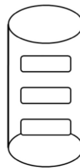
Fig. 3. PMMA cylindrical bar for placing TLD.
