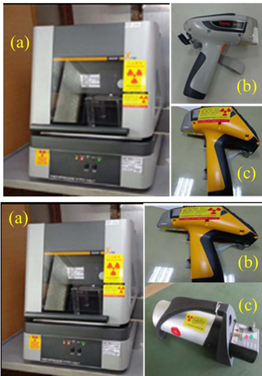
Fig. 1. Example photos of (a) cabinet-type X-ray equipment and (b) and (c) portable X-ray devices.
