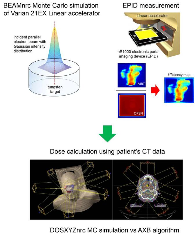
Fig. 1. The MBMC simulation setup.
