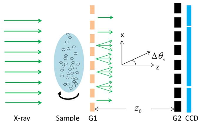
Fig. 1. The diagram of X-ray dark-field computed tomography using a grating interferometer.
