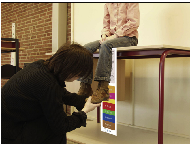
Fig. 1. Evaluation of Popliteal Height with the “Peter lower leg meter”.
