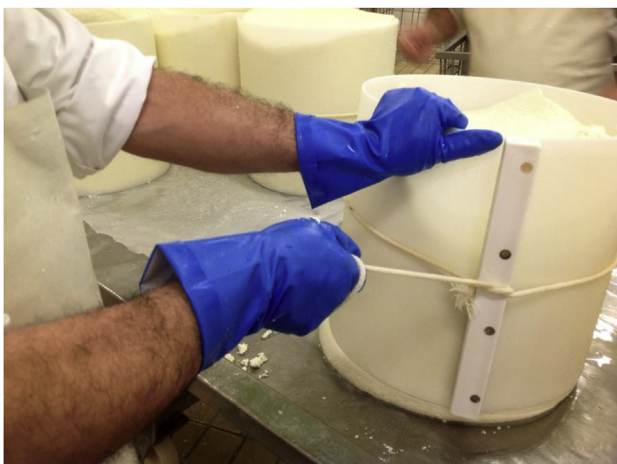
Fig. 1. A worker tightens a mold around a 25 kg Pecorino Romano cheese wheel.
