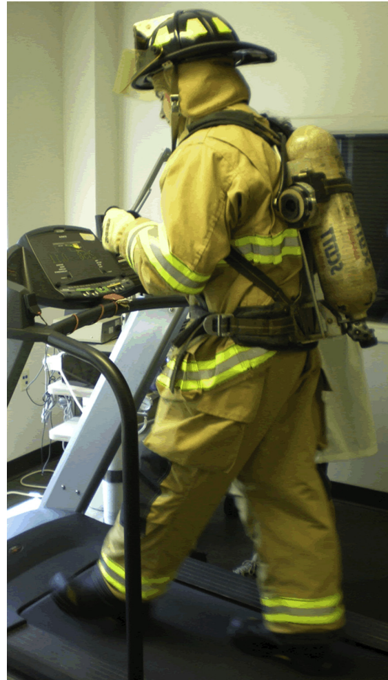
Fig. 1. During treadmill walking the participant wore the base layer (in this case cotton) under personal protective equipment, which included self-contained breathing apparatus.
