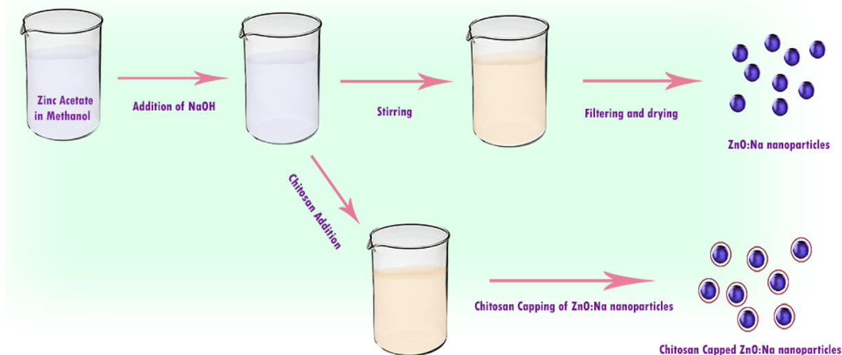
Fig. 1. Schematic representation of the synthesis of ZnO:Na nanoparticles by wet chemical method.
