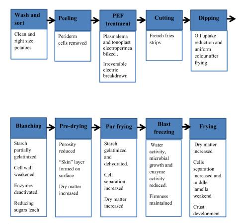
Fig. 1. French fry manufacturing process.
