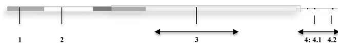
Fig. 1. SafeSpeed Carrier. Detailed outline of the SafeSpeed carrier and its components. The capillary where the oocytes are introduced is assembled into a main straw with a sealable rear-end and a slide cover for protection of the capillary during storage. 1: Sealable rear-end. 2: Labelling area. 3: Slide protector cover. 4.1: Sample placement marks, 4.2: Sealing mark.
