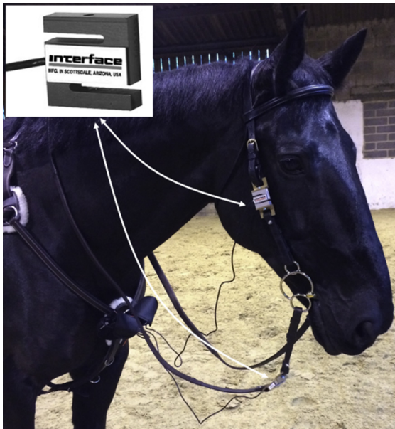
Fig. 1. S-beam mini force gauges (inset) included in the line of the reins and that of the leather strap cheekpiece (CP), here installed on the offside of the horse. The wireless transmitters are contained in adapted camera cases attached to the breastplate. The bit cheek shown is of the type B depicted in Fig. 2, and the mouthpiece is of a double jointed design.
