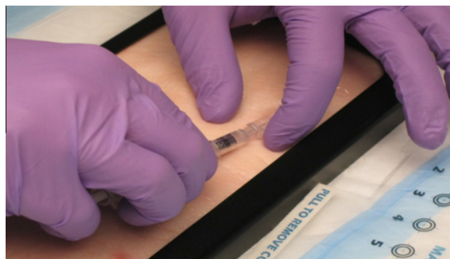
Fig. 1. Excised pig skin in custom frames preventing the skin shifting during the evaluation.
