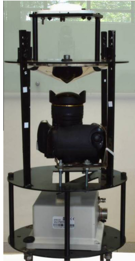
Fig. 1. Omnidirectional vision system composed of a wide-angle camera and a conic mirror. The system also has a double frequency SPAN-CPT/Novatel GNSS (Global Navigation Satellite System) receiver and an IMU (Inertial Measurement Unit) for direct image georeferencing.
