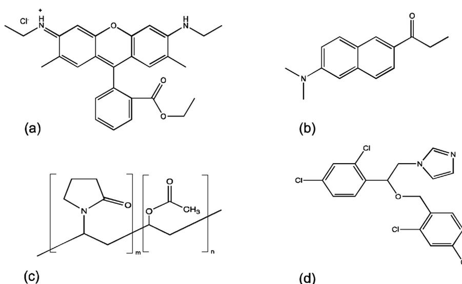
Fig. 1. Structures of the compounds used. Rhodamine-6G (R6G) (a), prodan (b), poly (1-vinylpyrrolidone-co-vinyl acetate) (PVPVA) (c) and miconazole (d).
