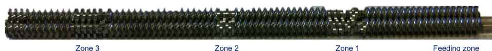
Fig. 1. Image of the twin – screw configuration used for the extrusion granulation process.
