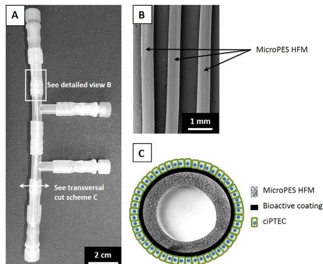
**Fig. 1.** Upscaled “living membrane”. (A) Picture of one module used for upscaled “living membrane” model. Three MicroPES hollow fiber membranes (HFM) within a housing composed of PE, PP and silicone parts, Luer Lock fittings and caps. (B) SEM image of three MicroPES HFM. (C) Scheme of a transversal cut of one “living membrane”. Not at proportional scale.
