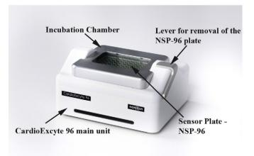
**Fig. 1.** The CardioExcyte 96 with incubation chamber, NSP-96 in recording position and hand lever for removal of the NSP-96. By using the incubation chamber, a constant temperature and humidity can be maintained without the need for a separate cell culture incubator. The use of the incubation chamber minimizes temperature changes when exchanging solutions, e.g. by media changes or addition of compounds.
