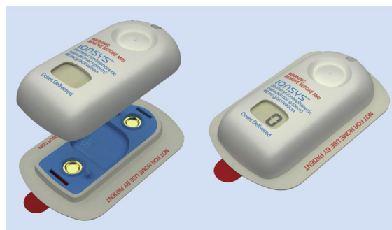
Figure 1. Illustration of the fentanyl iontophoretic transdermal system controller and drug unit and assembled system. The device is approximately the size of a credit card. The controller and drug unit are assembled by the health care professional immediately before the application. This figure is available in color online at www.jopan.org . Reprinted with permission from The Medicines Company (Parsippany, NJ).
