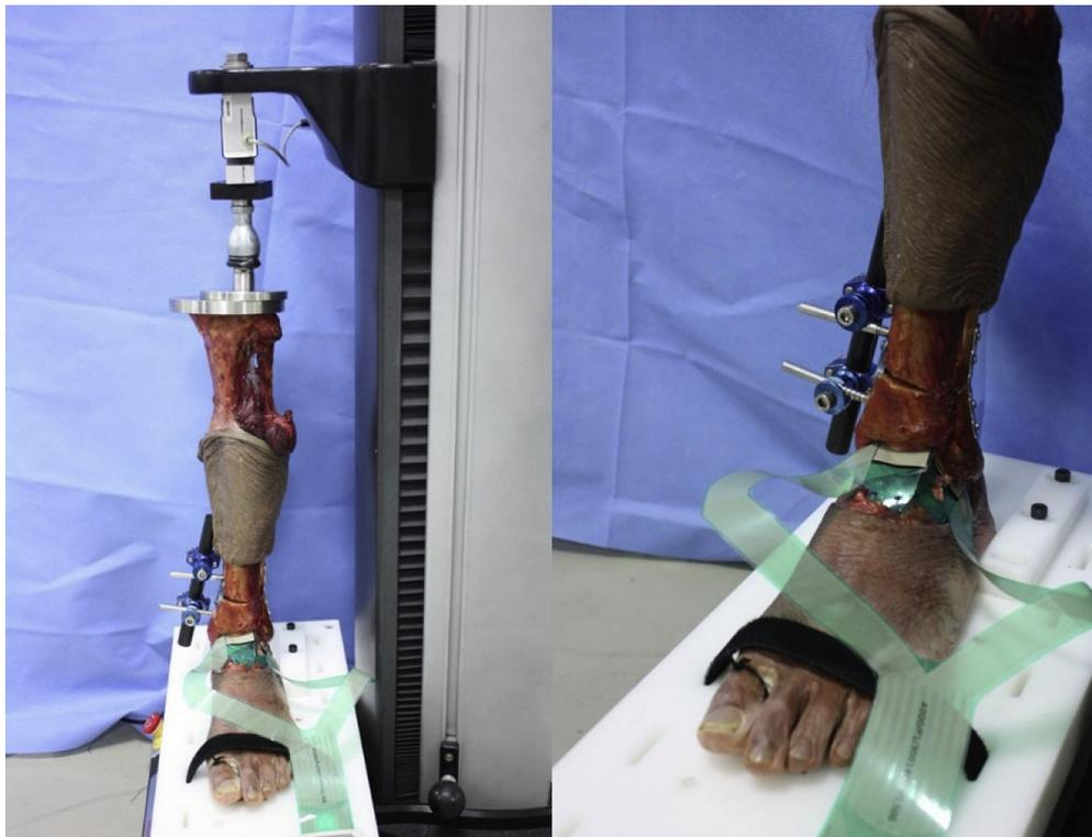
Fig. 1. Experimental setup. The specimen was fixed with the customized plate attached to the loading machine. Two identical, independent Tekscan pressure sensors were placed in the tibiotalar and talofibular joints, respectively.
