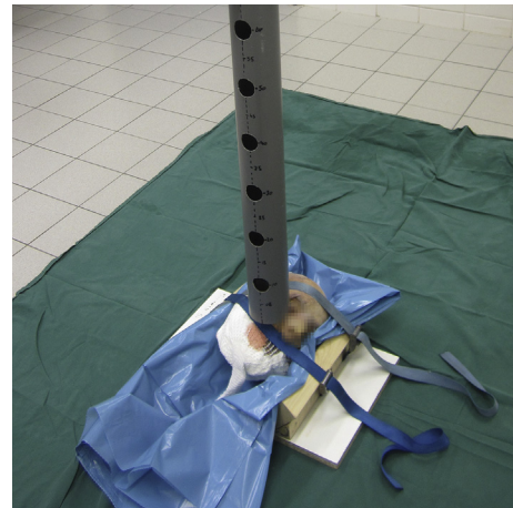
Figure 1. Infliction of the zygomatic fractures. The zygoma-orbital fractures were systematically inflicted on the cadaver head using 2 kg weights and a free fall impact. A 160 cm tube guided the weights to the malar eminence during a vertical drop.
