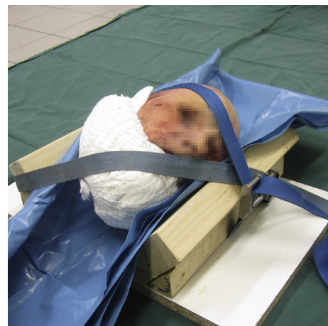
Figure 2. Placement of the human cadaver heads for the infliction of the zygomatic fractures. The cadaver heads were placed on a 52° wooden wedge to ensure perpendicular impact on the malar eminence. In the picture, the face was pixelized for ethical reasons.
